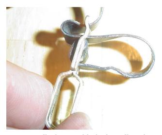
Figure 18 - Detail of control belt threading through clevis
