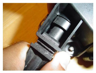
Figure 10 - Sliding out throttle cable
