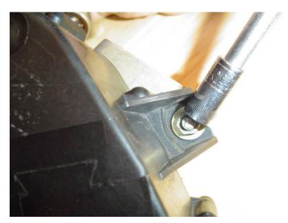
Figure 13 - Remove mounting plate nuts
