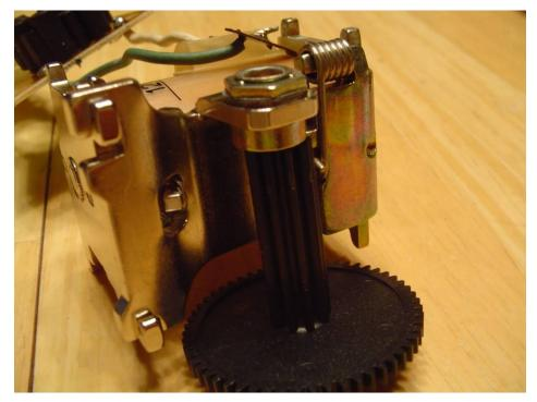
Figure 26 - Solenoid and drive engagement sprocket (partially reassembled)
