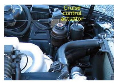
Figure 25 - Typical E34 mounting (non-540i)
