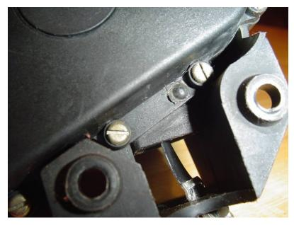
Figure 14 - Remove shell perimeter screws
