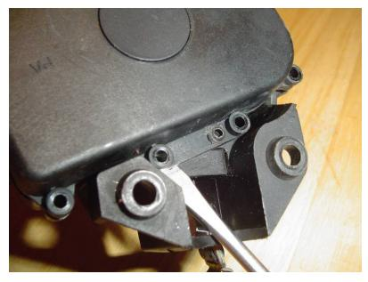
Figure 15 - Using screwdriver to separate shell halves
